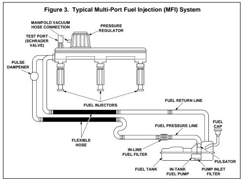
Some fuel injection systems **are not** equipped with a test port (Schrader valve). In some cases, these systems may be tested using the tee adapter provided with the tester:
